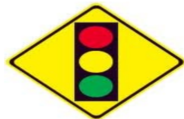
Figure 3-17. SIGNAL AHEAD Sign (W3-5).
